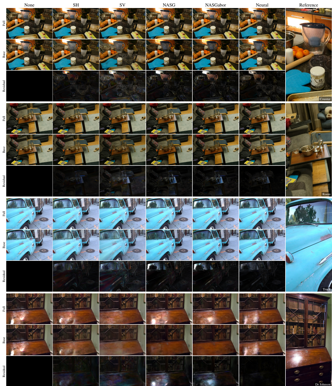
Figure 6. Base color and view-dependent residual, visualized as in Fig. 2, for a test view of four scenes. NASGabor achieves the best decomposition, with the residual limited to reflections such as those on the desk in Dr Johnson . The SV residual often also models diffuse appearance. The neural model incorrectly represents the highlight on the desk in Dr Johnson with the base color instead of the residual.
